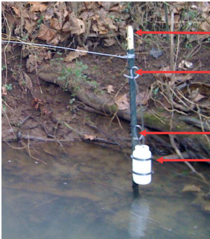
Figure 5: The typical passive sampler setup. The only time this setup was changed was if the stream bedrock prevented the installation of a fence post.
